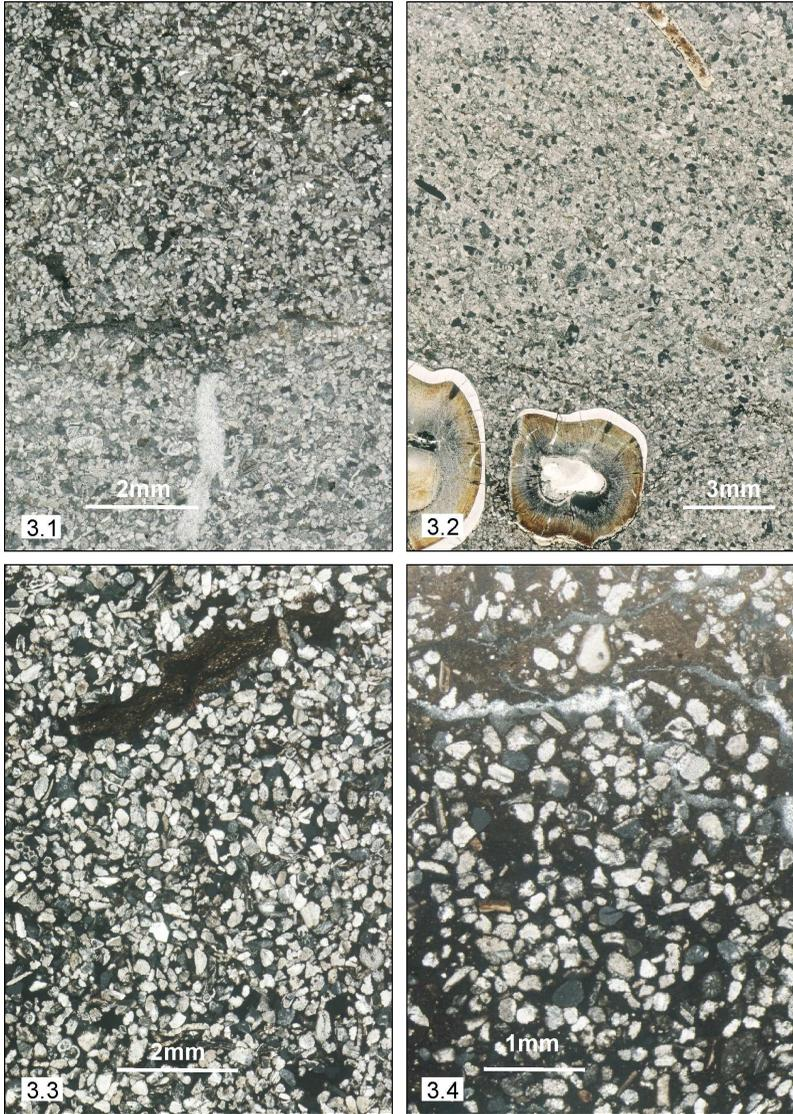
**Figure 3.1.** Scontrone Fossil Site section. Bioclastic packstone with large specimens of *Ammonia* (lower side) crossed by a vertical bifurcating spar-
