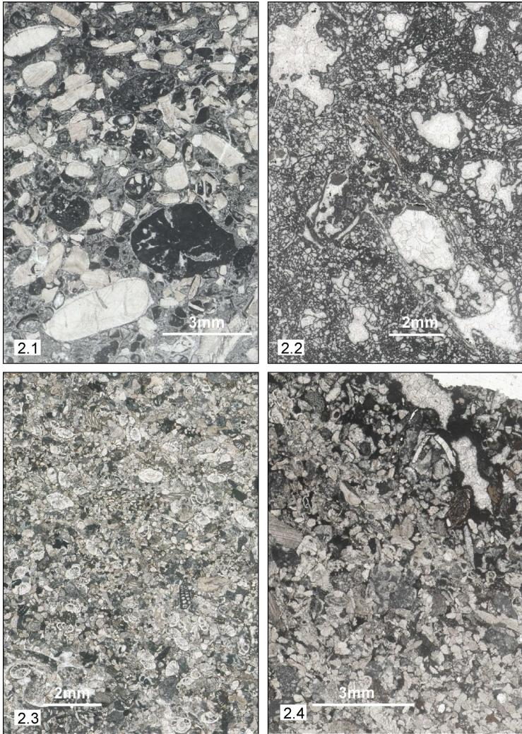
*Figure 2.1. Scontrone Cemetery section. Litho-bioclástico packstone with very well-rounded fragments of rudists (requienids) and oversized*
