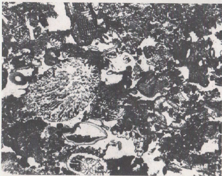
FIG. 8—Eocene shallow-water limestone from Malta E Escarpment, dredge 5 (2,786 to 1,958 m). Bioclastic grainstone/packstone with corals, bryozoans, brachiopods, and shell debris. Thin section, \times 4 .
