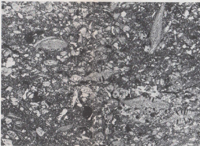
FIG. 10—Uppermost Oligocene calcarenite from Malta E Escarpment, dredge 6 (2,653 to 1,858 m). Bioclastic wackestone with Lepidocyclina , Amphistegina , and planktonic forams. Thin section, \times 5 .
