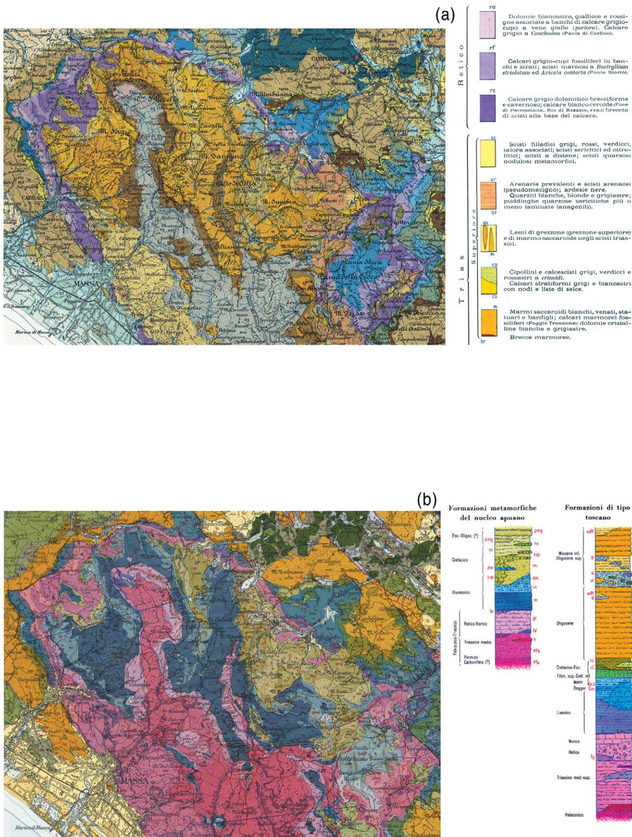
Fig. 5 - The two editions of the sheet 96 - "Massa" of the Geological Map of Italy at the 1:100,000 scale, by the Servizio Geologico Italiano. The first edition (a) is mapped by ZACCAGNA between 1879 and 1910 and is published in 1923. The second edition (b) is edited by TREVISAN *et alii* and is published in 1970.
