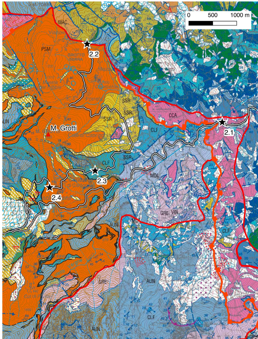
Fig. 34 – Sketch map of the area of Stops 2.1, 2.2, 2.3 and 2.4, modified from Puccinelli et al. (2010) and Conti et al. (2018). The thick red lines are low-angle normal faults, orange lines with barbs show the tectonic base of the Calcare Cavernoso.
