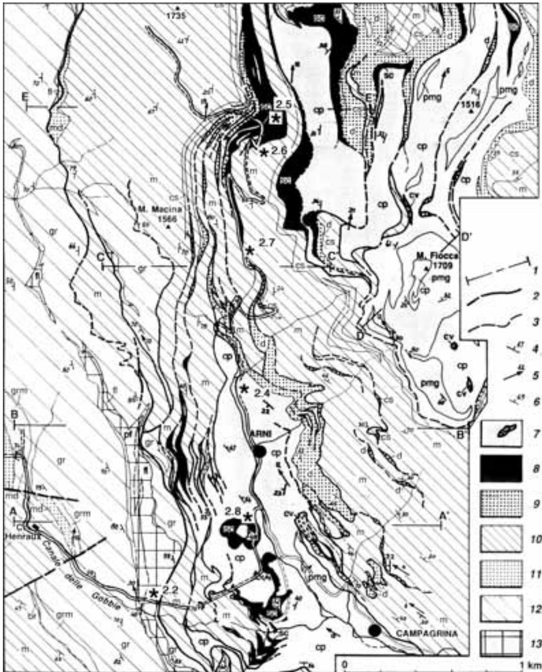
Figure 21 - Geological map in the Arni valley. 1: traces of sections of Fig. 22; 2: faults; 3: tectonic contacts; 4: D2 foliation; 5: D2 fold axis; 6: D1 foliation; 7: "Pseudomacigno" metasediments (pmg), calcschists (cp), "Calcare cavernoso" (cv); 8: "Scisti sericitici" phyllites (sc); 9: Cherts (d); 10: Calcschists (csc), cherty limestone (cs), marble (m); 11: Dolomitic marble (md); 12: Seravezza Breccia (br), "Grezzoni" dolomite (gr), "Verrucano (fV+Vr); Paleozoic phyllites (pf+fl).
