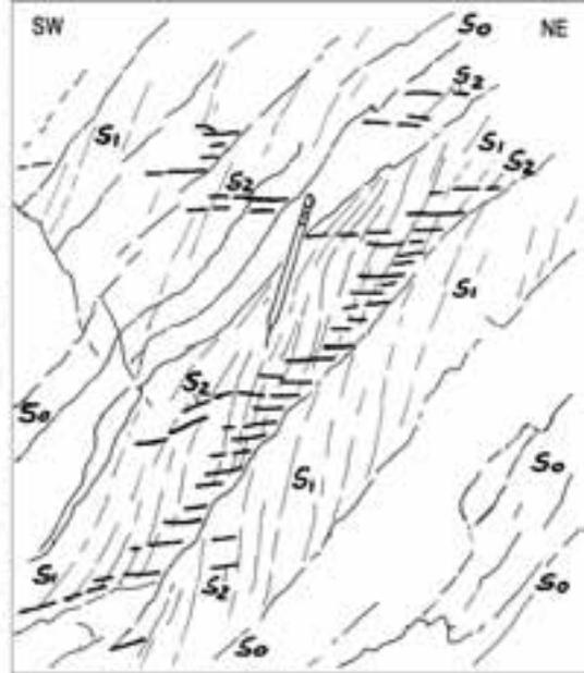
Figure 12 - S0, S1 and S2 interference in the road cut at La Maestà di Castelpoggio. S0-S1 relationships indicate a top-NE facing for D1 fold, S0-S2 relationships indicate top-SW facing for D2 fold.
