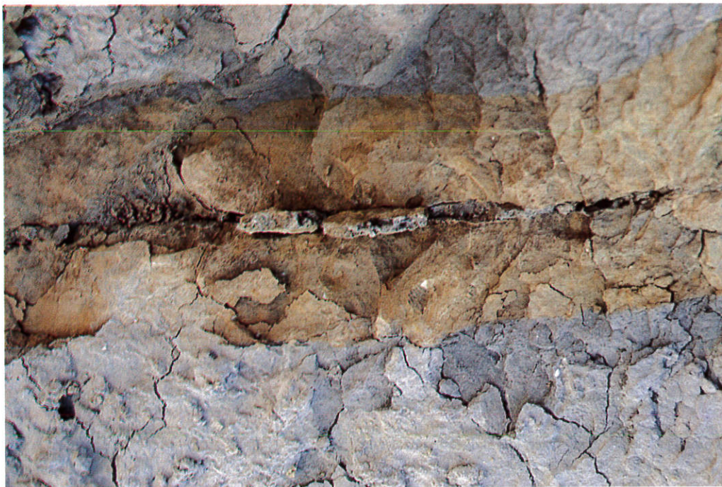
Photo 2 - Chalk large crystals filled fracture (Costalpino quarry).
