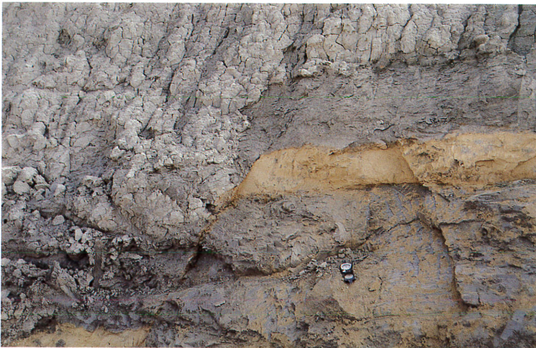
Photo 9 - Small throw normal fault in the quarry at Costalpino, with N140 strike in agreement with the fractures in the quarry. Note that the oxidation phenomena, which pervade the sandy layers, involve the fault plane.
